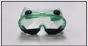
Figure 2: The goggle taped at the bottom avoids the subject looking in the downward direction.
