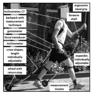
Figure 1: Cross-shaper, construction and measurement technique
