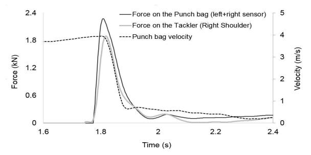
Figure 2: Example of forces measured on punch bag (black line) and tackler (grey line), and punch bag velocity (black dashed line), versus time.
