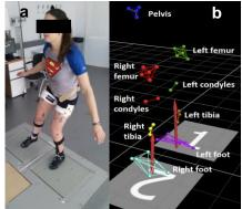
Figure 1: (a) A participant wearing reflective motion capture markers and EMG electrodes (results not presented); (b) Motion capture landmarks as displayed in Vicon Nexus software.
