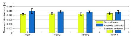
Figure 3: Mean distance between a reconstructed marker and the associated real marker and standard deviation over four throwing motion capture with the two methods
