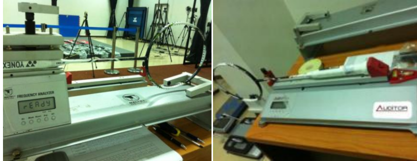
Figure 1: The validity testing: shaft stiffness and moment of inertia
