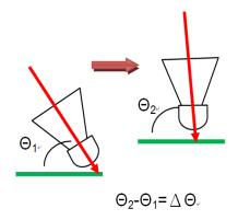
Figure 3: Shuttlecock tumbling angle definition.
