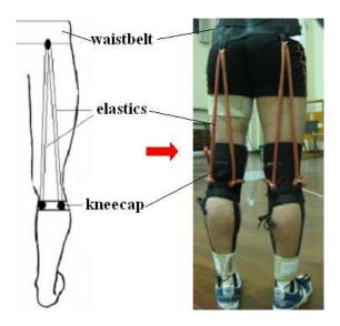
Figure 1: The demonstration of external muscle system.
