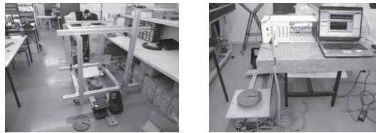
Figure 2: Setup for weight lifting and for calibration purposes.
