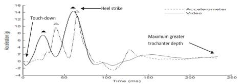
Figure 1: Sample tibial acceleration curve assessed via accelerometer (dashed) and video (solid). The triangles indicate the peaks (open = accelerometer; solid = video).
