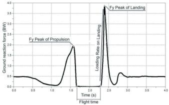
Figure 1: Variables analyzed for the vertical component of the GRF.
