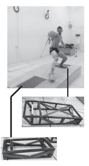
Figure 1: The structure of pitching mound. Two force plates were locked on these steel frames, then a wooden box covered it.
