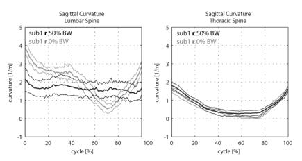
Figure 3. Sagittal curvature of the lumbar (left) and thoracic (right) spine of sub1. Mean and SD over 8 cycles. r 0% BW (grey), r 50% BW (black).
