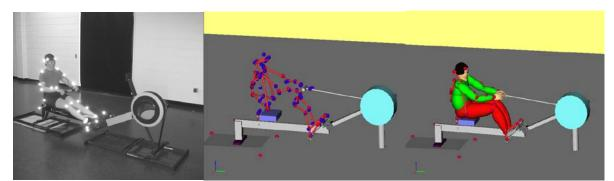
Figure 4: Process of data acquisition, transferring the movement data to the multi body system model, and reconstruction of the movement performing inverse kinematics.
