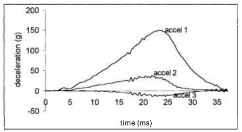
Figure 1- Deceleration signals from the three orthogonally arranged accelerometers (accel 1, 2, 3) from a drop on the Pinetree green mat.
