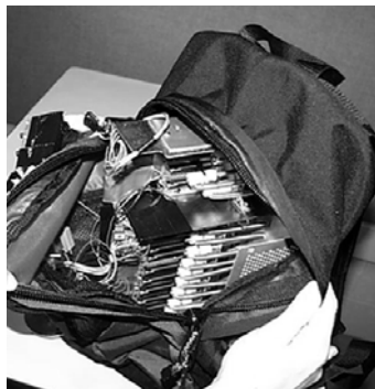
Figure 3 - Inside of the data logger backpack
