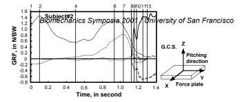
Figure 2- Changes of GRFs acting on the pivot and stride feet in Subject#2. Shin lines with solid, broken and dotted shows the vertical (Z), anterior-posterior (Y) and rightleft (X) GRFs for the pivot foot, and also thick lines for the stride foot. Each number for the vertical lines corresponds to that for the stick figures of Subject#2 in Fig. 1. Force data are normalized with body weight (BW).
