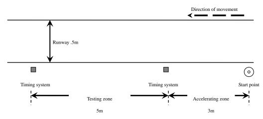
Figure 1: Experimental setup of overground running, i.e. tartan, grass and treadmill
