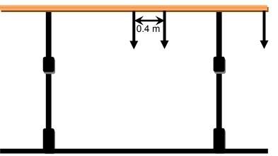
Figure 1: Location of the Calibration points on the bar.
