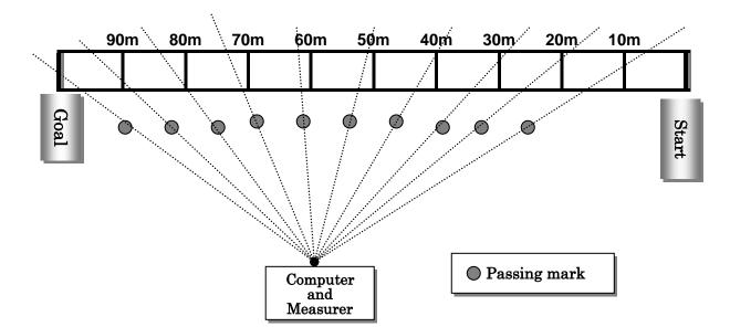
Figure 1 - The experimental straight lane for the measurement of the 100m dash is shown. The lane was divided equally into 10 sections. Each passing mark was placed on an extension line from the measurer to a passage point of each section.
