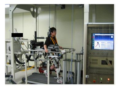
Figure 5: Developed robotic gait trainer
