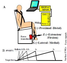
Figure 1. Schematic representation of experimental setup (A) and target force trajectories (B) in the present study
