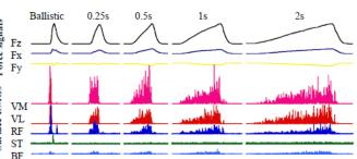
Fig. 2. Representative recordings of three components of force signals and surface EMG activities on thigh extensor and flexor muscles at five different force rise times
