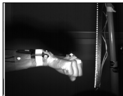
Figure 1: Scheme of the measuring station for complex 1 (left), high speed record of the hand with markers and acceleration sensor before reaching the target (board)
