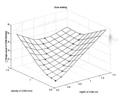
Figure 2 Simulation of the stability of loaded walking at slow walking.
