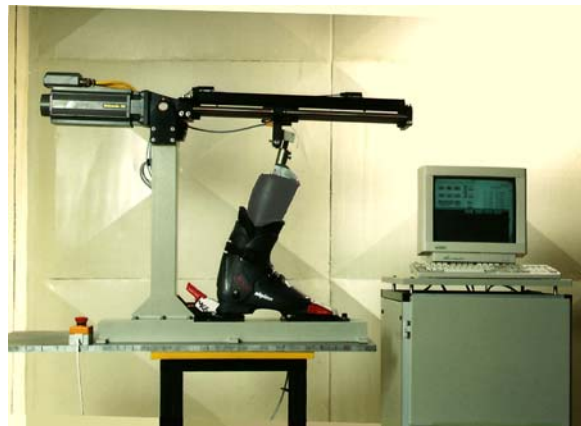
Fig 4. Manipulator for testing alpine ski boots
