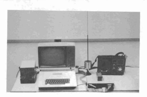
Figure 5. Signal reception, conditioning and recording instrumentation; clockwise from centre - receiving antenna, FM receiver, decoder, and microprocessor.
