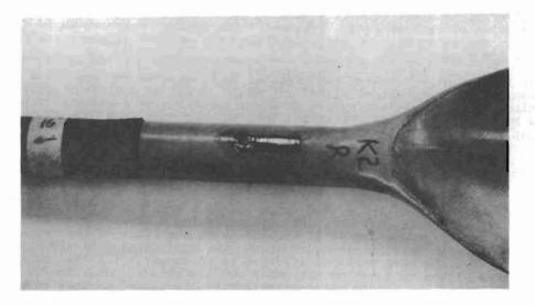
Figure 4. Strain-gauge location - kayak paddle.
