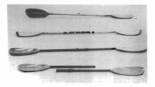
Figure 3. Instrumented kayak paddles: top - solid wood; second - wood adjustable; third and bottom - carbon fiber, adjustable, hollow core.
