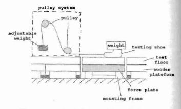
Figure 1 - mechanical slip resistance test setup
