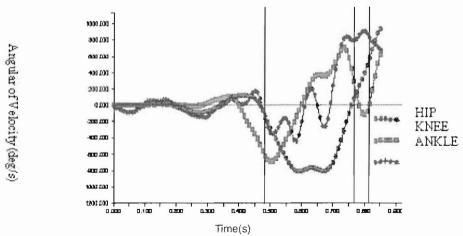
Figure 2: Angular velocities of hip, knee and ankle joints from a selected subject.
