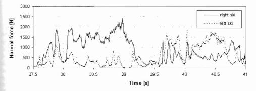
Figure 2: Force component normal to the ski surface measured by Kistler® force sensors.
