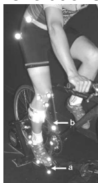
Figure 2: Detail of metallic sticks on the pedal (arrow a), and tibia (arrow b).
