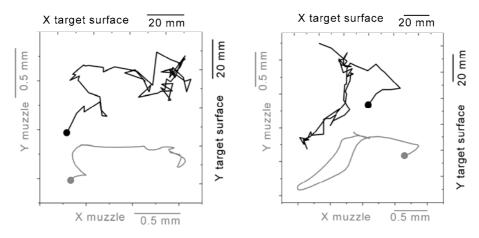
Figure 3: Sample 2D-trajectories and hits of two different shots. The muzzle trajectory in X-direction is shown mirror-inverted. Note that relative trajectories are obtained only.
