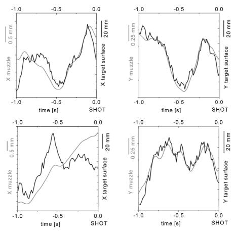
Figure 4: Sample trajectories of two shots as a function of time. Top: example shot for a high similarity in both X- and Y-direction. Bottom: example shot for a poor similarity in X-direction.
