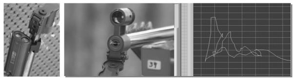
Figure 1: Left: optoelectronic feedback system Noptel. Right: video-based system. The plotted line in the diagram represents the trajectory of the muzzle obtained from the video (Baca & Kornfeind, 2006)
