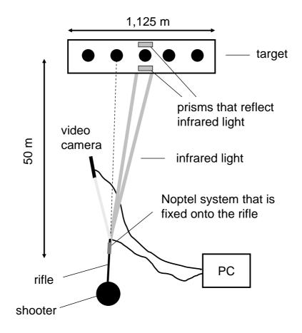
Figure 2: Schematic assembly of the system
