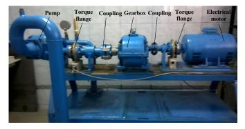
Figure 1. Main components of the test stand [13]
