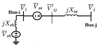
Fig. 1 — UPFC representation using voltage sources.
