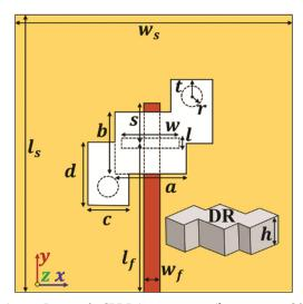
Fig. 1 — Proposed CPDRA geometry ( $l\_s = w\_s = 80, a = 14, b = 12, c = 8, d = 12, h = 10.5, l\_f = 40, w\_f = 1.6, s = 7, w = 9, l = 1.2, t = 4, and <math>r = 1.8$  (all dimensions are in mm).
