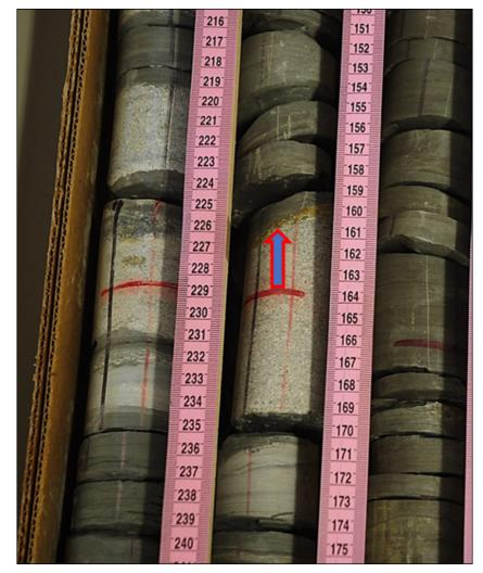
FIGURE 5. Core segments near Lexington-Point Pleasant contact (arrow), showing eroded and corroded nature of the contact with hematite (oxidized pyrite) coating the contact. Note the calcarenitic limestones and interbedded dark shales that comprise upper parts of the Lexington and the gray-brown shales that comprise the overlying Point Pleasant. Scale in centimeters. OGS core 2984, Butler County, southwestern Ohio, Well No. 52, at a depth of 158 m (517 ft) below the surface.
