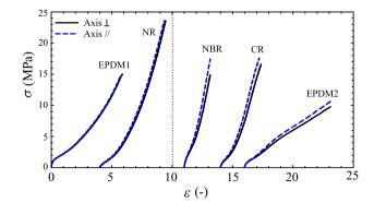
**Fig. 8** Nominal stress–strain response under uniaxial deformation for specimens aligned perpendicular to or parallel to the rolling direction (NBR, CR and EPDM2), or for compression-moulded specimens (EPDM1, NR), two orthogonal directions aligned with the mould axes. Offsets for clarity: EPDM1=0; NR=4; NBR=11; CR=14; EPDM2=16
