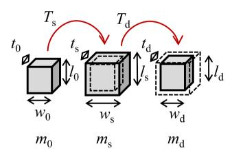
Fig. 5 Linear dimensions recorded at different stages of the swelling and drying procedure
