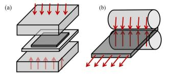
Fig. 2 Schematic representation of the manufacturing processes of  ${\bf a}$  compression-moulding and  ${\bf b}$  sheet rolling by calendaring
