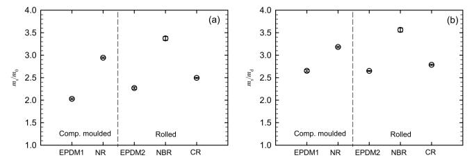
Fig. 7 Mass swelling ratios, a relative to the pre-swelling state; b relative to the post-swelling dried state. Data based on four specimens (±1SD)
