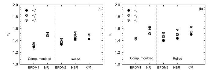
**Fig. 6** Dimensional swelling ratios, **a** relative to the pre-swelling state,  $\alpha'_i$ ; **b** relative to the post-swelling dried state,  $\alpha_i$ . Data based on four specimens ( $\pm 1$ SD)
