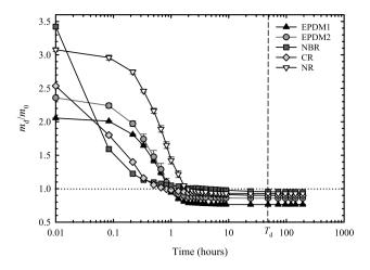
**Fig. 4** Drying mass ratio as a function of time during drying experiments on specimens swollen for 48 h. Initial swollen mass ratio predrying is shown at a representative time of 0.01 h. Dashed line indicates the drying time (48 h) used in subsequent experiments; solid lines are a guide to the eye
