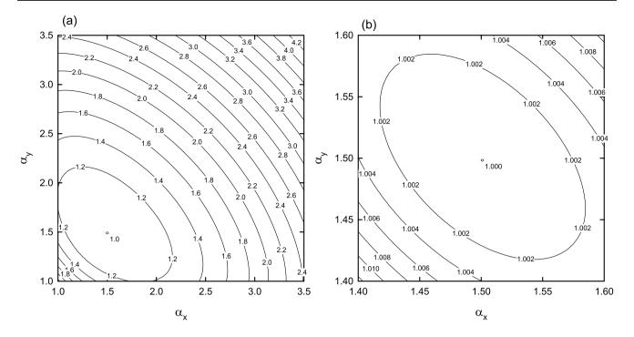
**Fig. 1** a Contour plot of the ratio  $\frac{\overline{M}_{c}^{\text{minor}}}{\overline{M}_{c}^{\text{plory}}}$  between the molecular weight between cross-links obtained using a set of anisotropic linear swelling ratios  $\alpha_x$ ,  $\alpha_y$ ,  $\alpha_z$  (Eq. (17)) and the molecular weight between cross-
