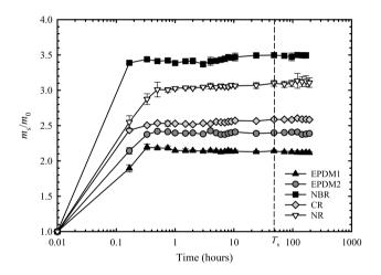
**Fig. 3** Swelling mass ratio as a function of time during swelling experiments. Initial mass ratio of unity (pre-swelling) is shown at a representative time of 0.01 h. Dashed line indicates the swelling time (48 h) used in subsequent experiments; solid lines are a guide to the eve
