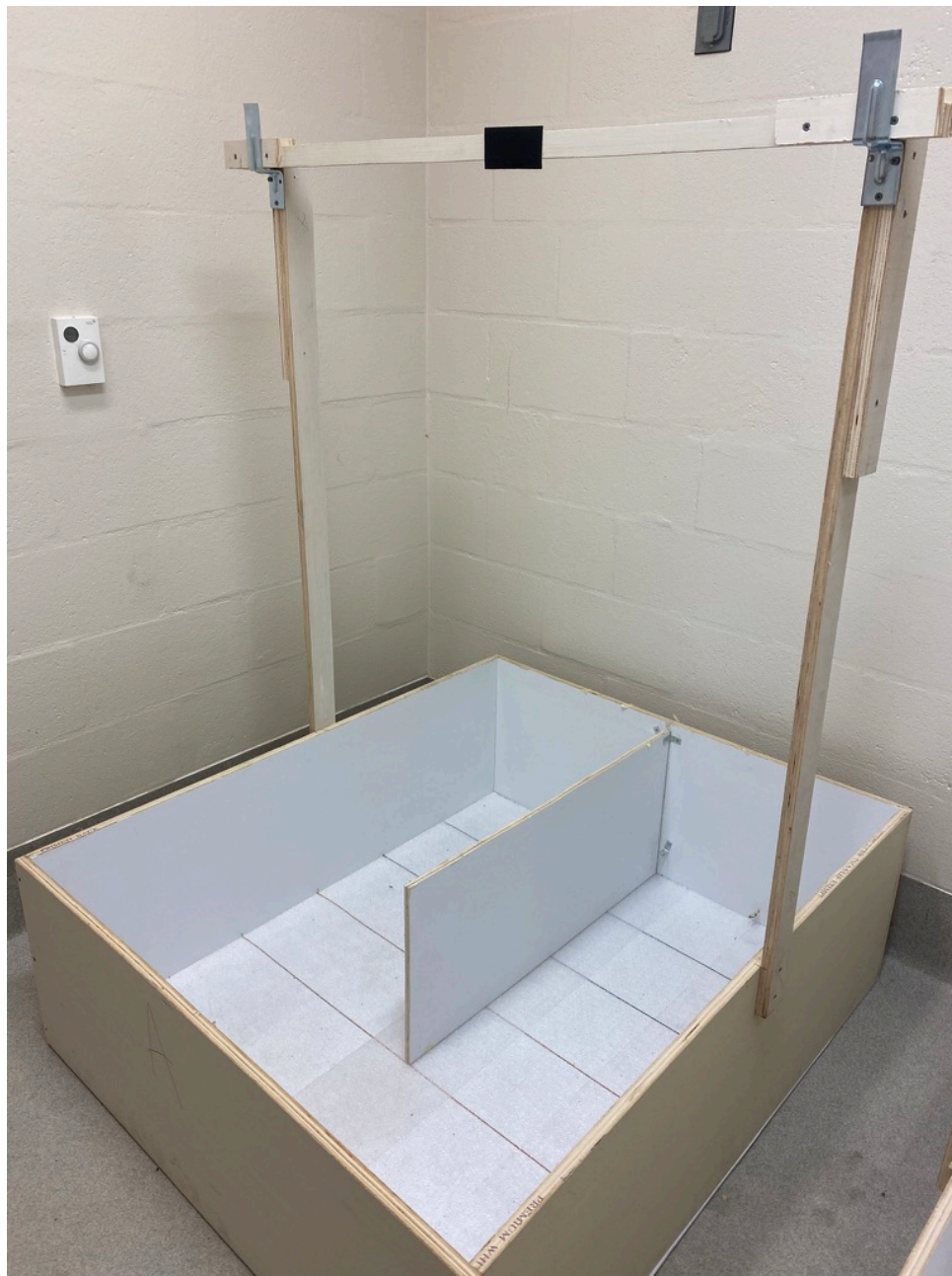
Figure 1. An arena set up for the combination trial. The video camera was mounted to the black Velcro attached to the plywood bar and plugged into the wall outlet for all trials.
