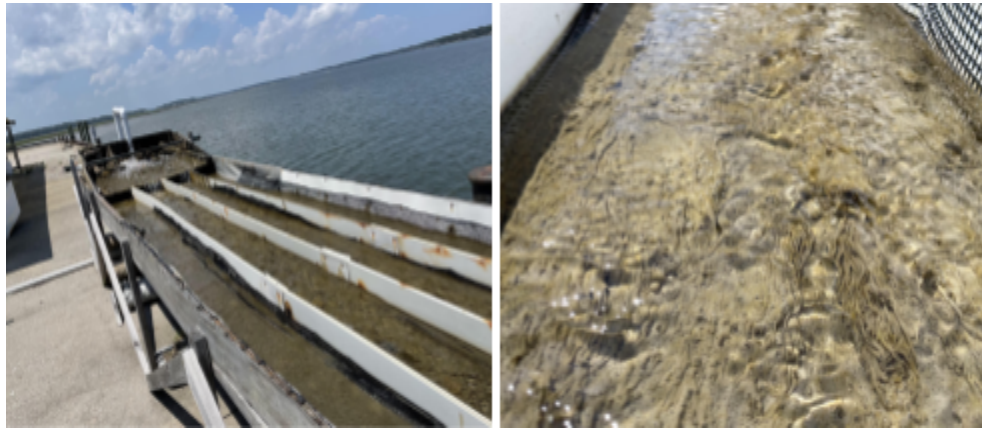
Figure 1. Algal Turf Scrubber (ATS) system at Priest's Landing docking site showing the flowways covered in algae and other benthic marine organisms.
