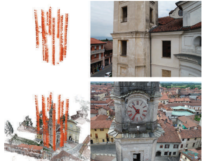
Figure 3. UAS acquisition scheme (left) and examples of acquired images (right).
