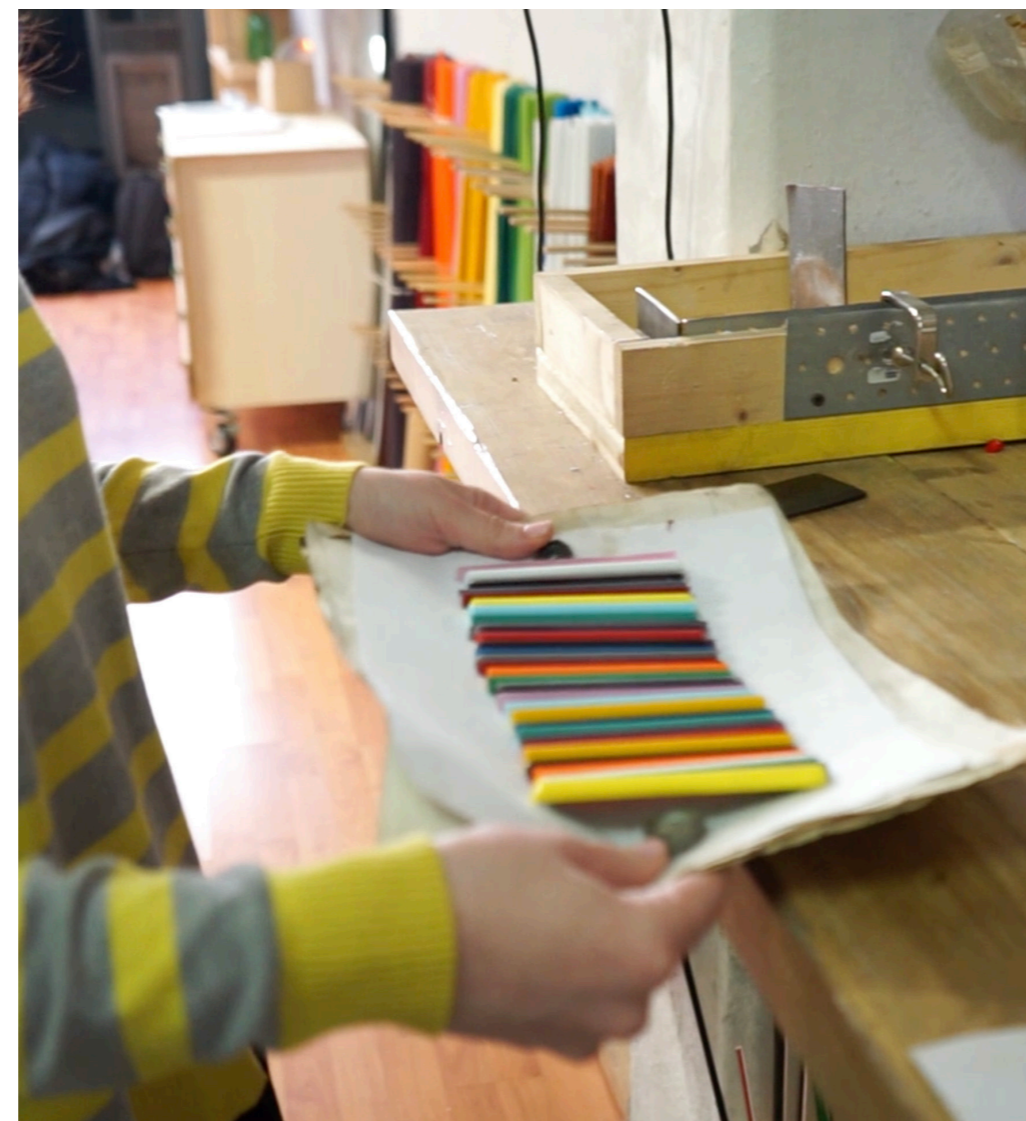
Figure 3. A workshop's participants personally arranged the rods in a colour combination of choice. Then the set is placed in the area dedicated to the heating of the glass.
