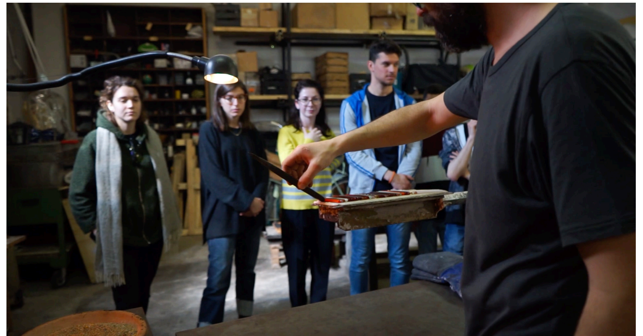
Figure 4. The glass master giving a demonstration to the workshop's participants of the first step for the creation of a vase. The combined rods are placed on a ceramic plate to be rolled-up and then blown to get the final shape.
