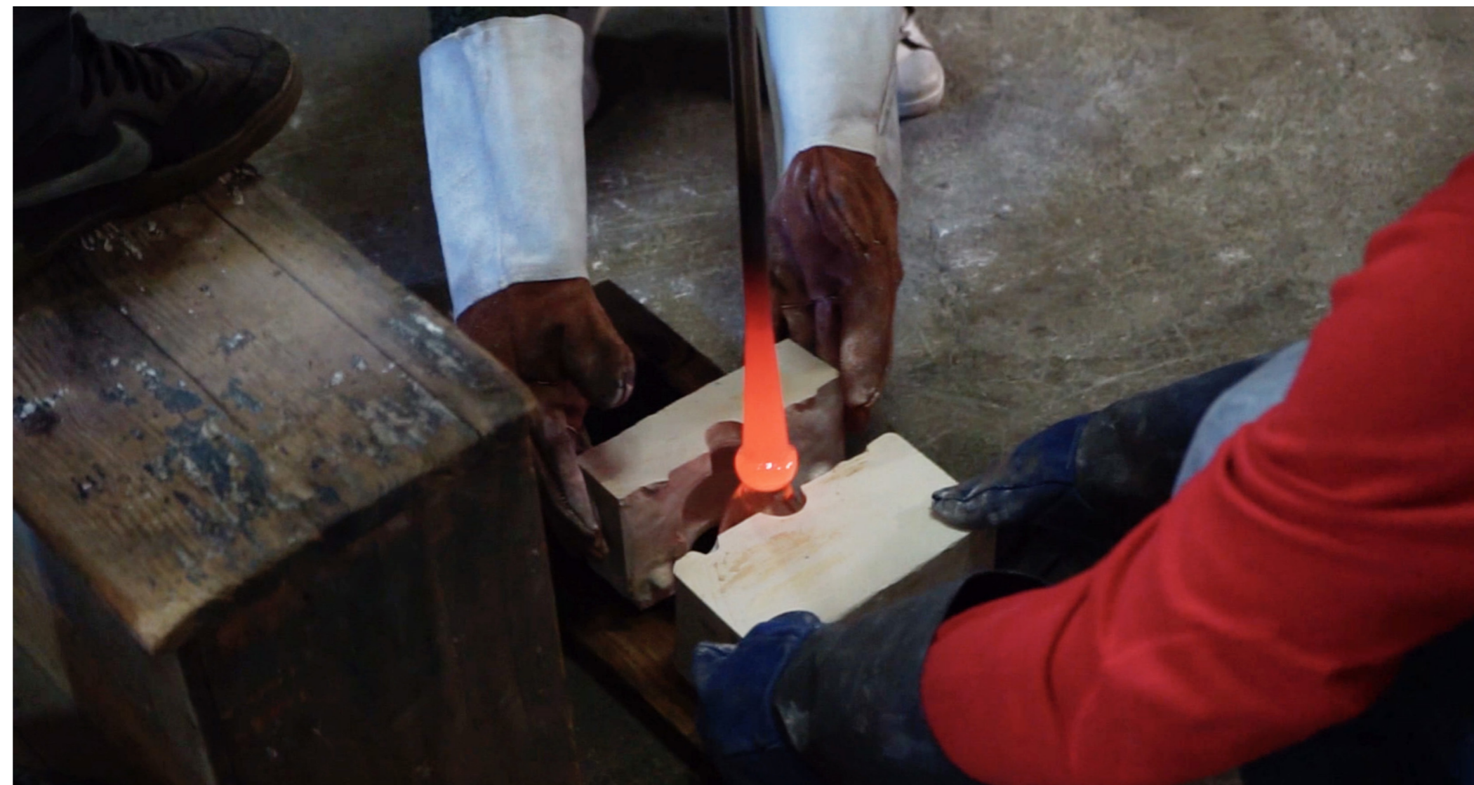
Figure 5. Two students collaborating to remove the blown object from the mould. Particular precautions must be taken during this step as the material is still extremely hot and delicate.
