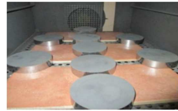
Fig. 7. Specimens of heat treatment in the oven
