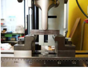
Fig. 19. Transversal break test device (TRS)
