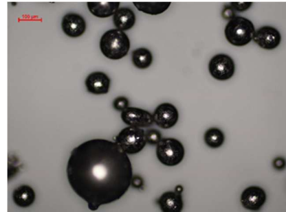
Fig. 4. Iron and silicon alloy with a spherical shape
