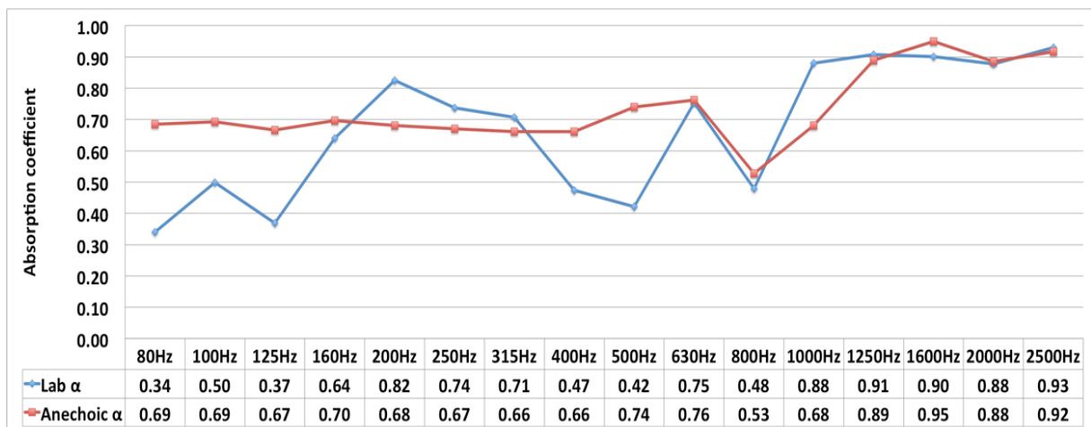
Figure 9: Absorption coefficient of tea-bag panel measured in anechoic chamber and laboratory condition using Impedance gun.
