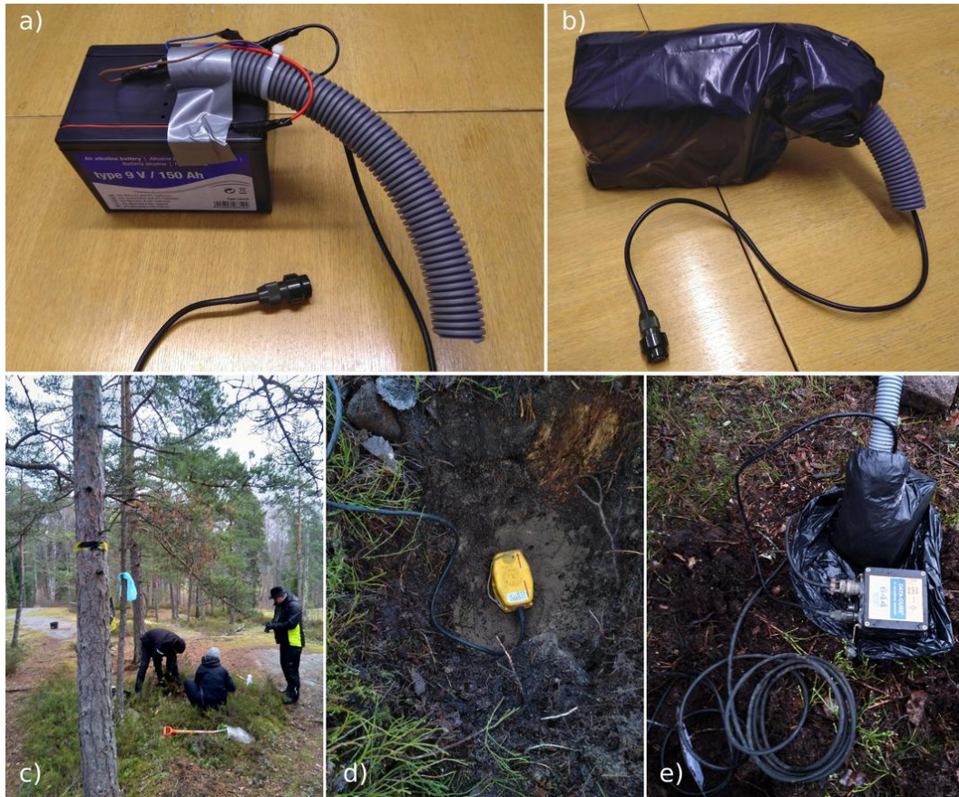
Figure 4. Installation impressions. (a,b) The air-alkaline batteries were prepared in a water-proof, compact, and inexpensive packaging with sufficient air-flow. The batteries were wrapped in plastic bags with a hose attached close to the air-holes at the top of the battery. (c) A typical installation site in the suburban Helsinki capital area. Most stations were installed on bedrock outcrops in a decimeters-thick organic soil or peat layer. (d) We used sand for better coupling of the geophones. (e) The batteries and recorders were placed in a shallow hole and camouflaged. Photographs by A. Rintamäki.
