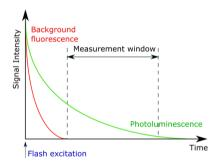
Figure 11. Time-gated luminescence intensity
