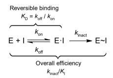
**Scheme 2**. Two-step mechanism of covalent inhibition between inhibitor (I) and target enzyme (E)
