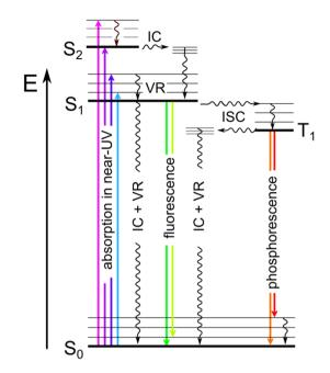
**Figure 7.** Jablonski's diagram, displaying the different molecular states ( $S_0$  – the ground state;  $S_1$ ,  $S_2$ , and  $T_1$  – excited singlet and triplet states) and photophysical processes – absorption, internal conversion (IC), vibrational relaxation (VR), fluorescence, intersystem crossing (ISC), and phosphorescence. Thicker and thinner vertical lines represent the electronic energy minimums and vibrational energy states, respectively [Lakowicz 2006].
