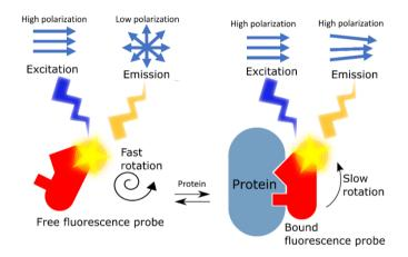
Figure 10. Principle of fluorescence anisotropy
