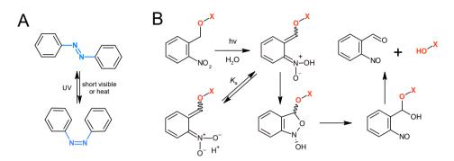
Figure 8. Reaction mechanisms of photosensitive compounds. (A) Reversible azobenzene type photo-switch. (B) Principal reaction mechanism of irreversible nitrobenzene type photolysis [Klán et al. 2013].
