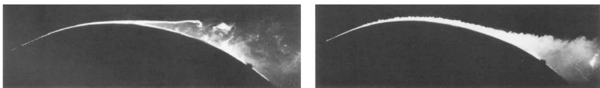
Fig 1.11. Boundary layer: laminar (left) and turbulent (right).
