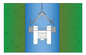
Fig. 1. The mechanism of the trash trap.
