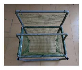
Fig. 7. Trash trap to collect diverted trashes.
