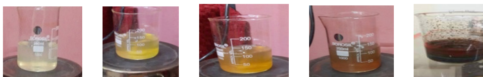
FIGURE 2. Colour changing process from pale yellow to Red-Brown
