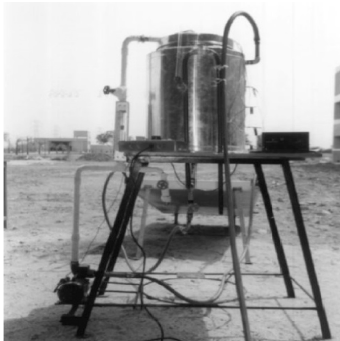
FIGURE 6. Experimental setup of combined storage with use of solar collector (Nallusamy et al. 2007)
