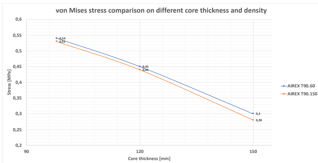
Figure 12: von Mises stress comparison on different core density and thickness [6]
