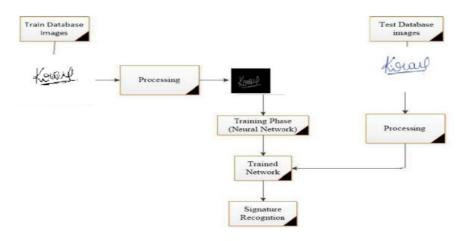
Figure 3.4.3: Image Processing Method.
